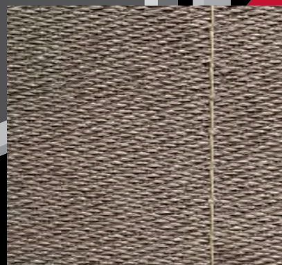
Curtain is constructed of a stainless steel wire reinforced glass fabric
